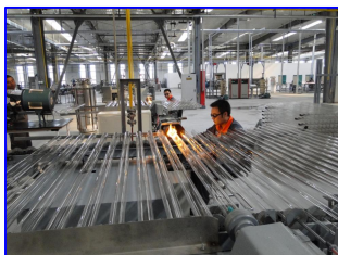
Inserting copper pipe (Top) into the glass tube and sealing of the vacuum tube (Bottom)
